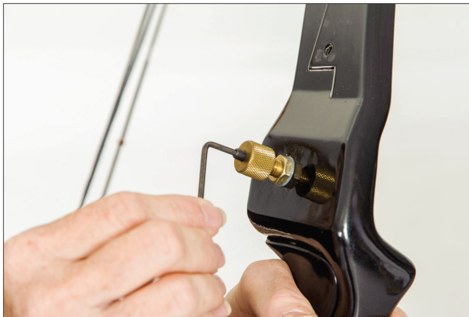
Figure 8.9 Adjusting the plunger tension.
