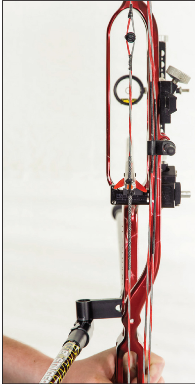
Figure 8.15 A shoot-through rest that is a true center-shot bow with a single piece of metal with a V notch in which the arrow rests.
