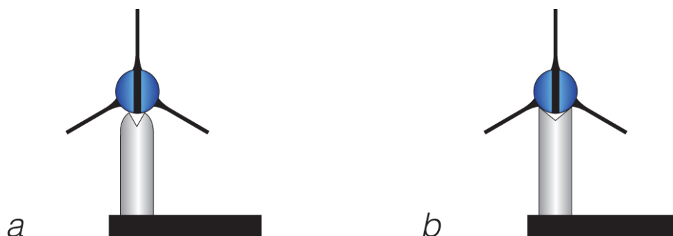
Figure 8.16 Shoot-through rests must provide good vane clearance: (a) good vane clearance; (b) poor vane clearance.
