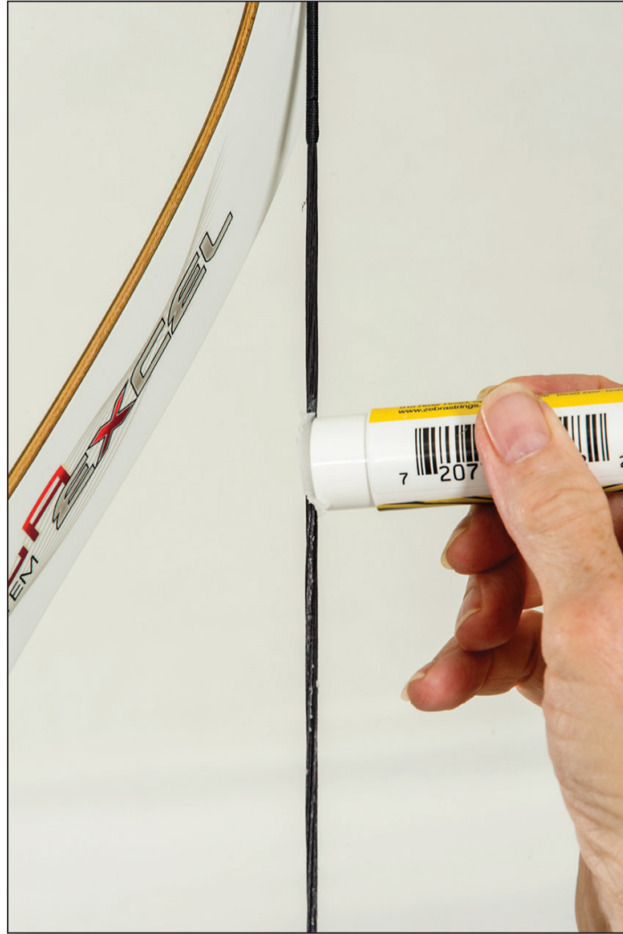
Figure 8.29 Waxing your bowstring minimizes fraying and protects it from moisture.
