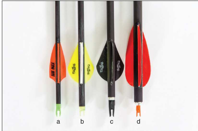
Figure 8.3 Various nock and fletching styles. Note that nocks can be attached directly to the swaged end of an aluminum arrow, inserted directly into the shaft, or attached to an insert or bushing.
