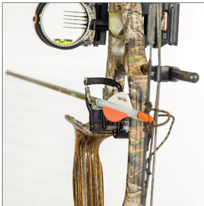
Figure 8.11 A drop-away rest. The rest drops down when the cables contact the plunger on the arrow rest assembly so that there is no contact with the arrow fletching as the arrow clears the bow handle.
