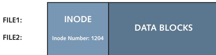
Figure 4-1 The structure of hard-linked files
