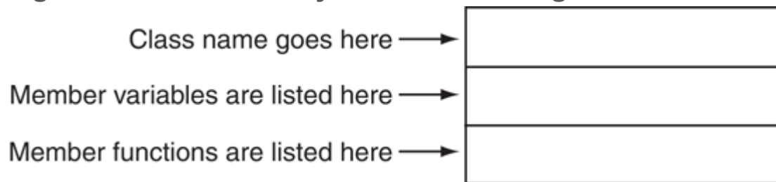
Figure 13-18 General layout of a UML diagram
